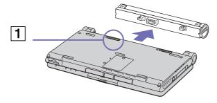
You may lose data if you remove the battery pack while the computer is on and not connected to the AC adapter or if you remove the battery while the computer is in **Standby** mode.
